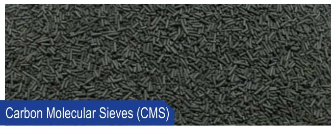
Carbon Molecular Sieve (CMS) is a new-style non-polarity sorbent. At room temperature and with varying pressure, CMS absorbs nitrogen and separates oxygen from the air.
